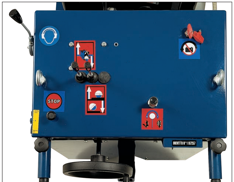
VDAI Saw: view of control panel with automatic forward/backward advancement lever; lever for lowering and raising the cutting blade; knob for adjusting the advancement speed and other controls. This photo shows the handwheel of the mechanical drive control device.
